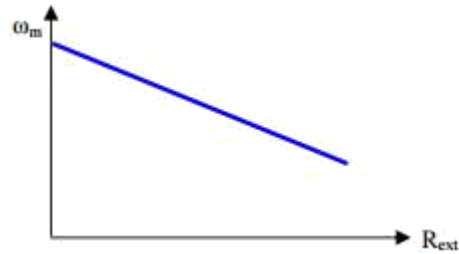
Fig. 12: Variation of speed with external armature resistance
