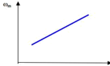
Fig.8. Variation of speed with applied voltage
