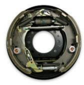
This type of Duo-servo type drum brake we were used in our car .Duo-servo type drum brakes are an improved version of twin leading construction, where two brake shoes are linked.
