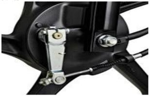
A drum brake is a brake in which brake shoes with ling (friction material) attached to them is pushed by hydraulic pistons against the inner surface of a drum rotating together with the axle.
