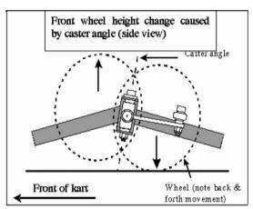
Castor angle is the angular displacement of the kingpin axis from the vertical axis of the vehicle measured in the longitudinal direction. It is the angle between the pivot line(in a car – an imaginary line that runs through the center of the upper ball joint to the center of the lower ball joint) and vertical.
