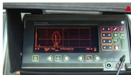
Fig 7.3: Ultrasonic testing flaw detector indication
