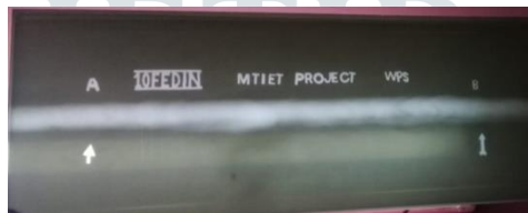
Fig 7.5: Radiographic film of Existing Parameters
