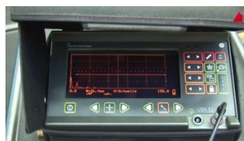
Fig 7.7: Ultrasonic testing flaw indication showing less flaws
