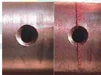
Fig5.4 workpiece performing magnetic particle testing
