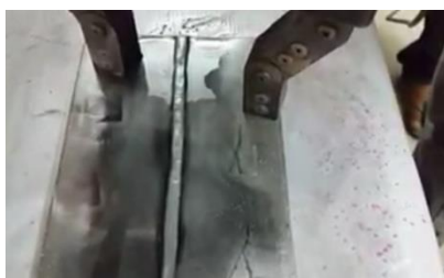
Fig 7.8: Porosity indications by particle
