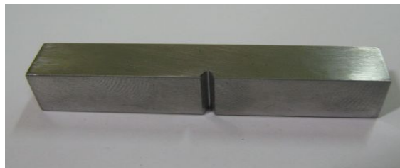
Fig. 5. Showing impact toughness test Specimen welded dual phase steel
