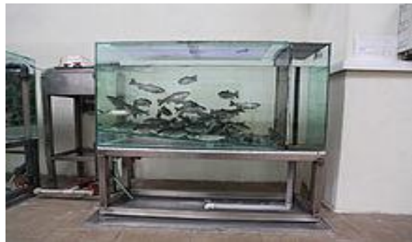
Fig 3.3: Rainbow trout are often used in water purification plants to detect acute water pollution.
