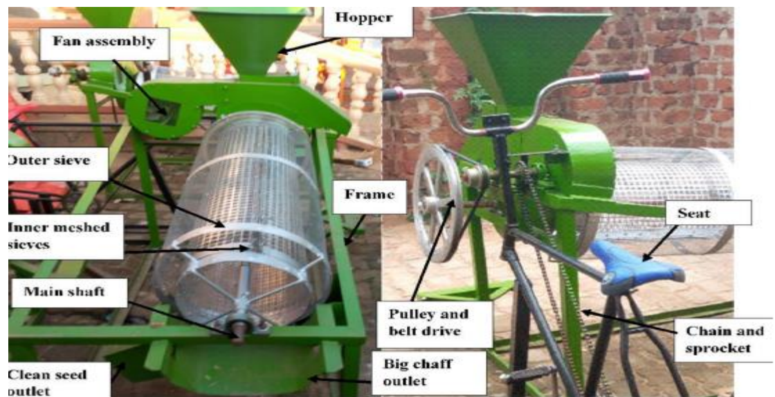
Fig 3.2: Assembly of the Pedal Operated Seed Cleaner
